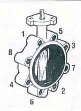
clearance for valve installation. The valve should be in the closed position when being placed between flanges. The valve should be operated to assure that no binding or interference is taking place. Flange bolting should be tightened gradually in a crisscross manner according to the illustration at right. Bolting should then be tightened sufficiently to prevent loosening of the joint.
