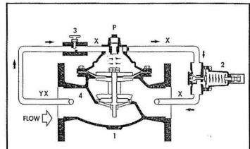
Flow Direction Shown: Under The Seat Optional 'R' Flow, Over The Seat
