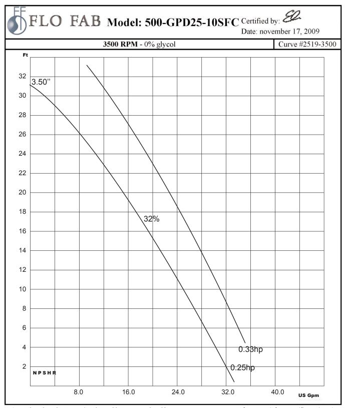
Curves based on shop test using clear cold water on a closed loop system at a temperature of not over 85°F at specific gravity 1.0
