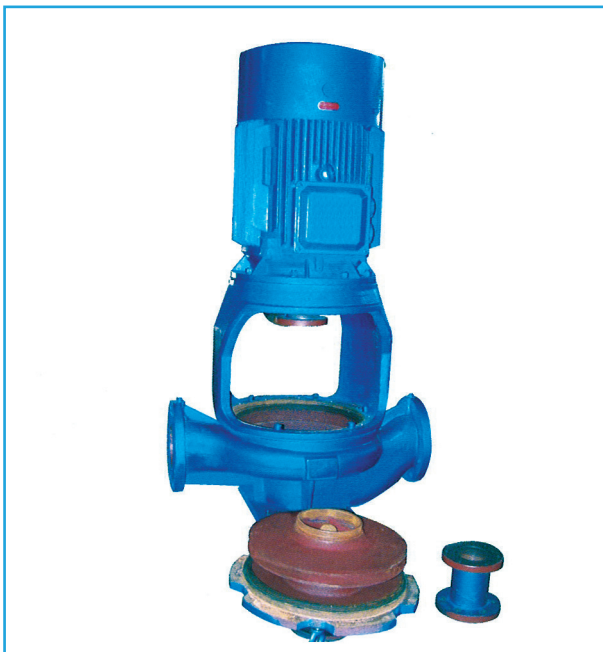
Take out the rotor components
