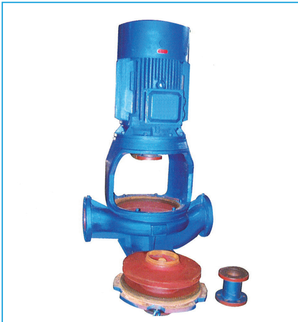
Take out the rotor components
