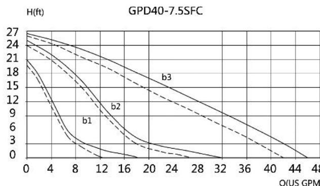
"— without check valve, "----"with check valve
