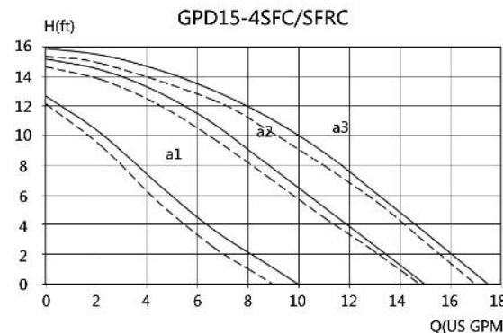
"— without check valve, "----"with check valve"
