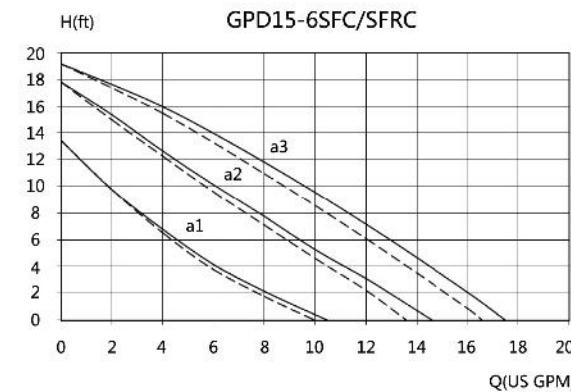
"— without check valve, "----"with check valve"
