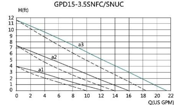
"—" without check valve, "----"with check valve
