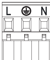
Figure 6: Pull-out terminal board for supply
