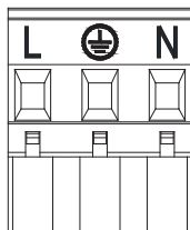
Figure 6: Pull-out terminal board for supply
