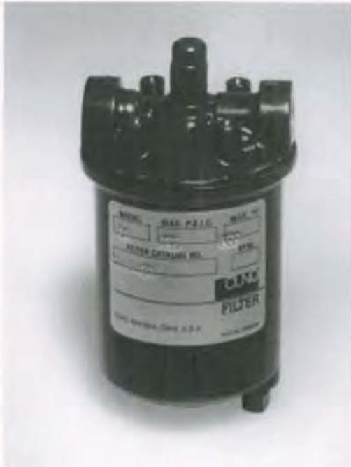
The 1A1 MODEL Cartridge Filter Housing is an all-metal, two-piece housing, featuring centerpost-type construction. The 1 A1 Model has a maximum operating temperature and pressure of 125 psig at 200°F. The 1A1 Model Cartridge Filter Housing has flow rates to up to 6 Gallons Per Minute (GPM).
